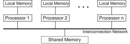
**Figure 2. Shared Memory Multiprocessor System Structure**
